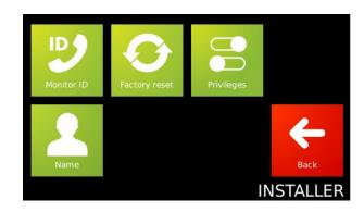
**Enter monitor ID** - This option is used to set up the Monitor ID. See Configuration.
