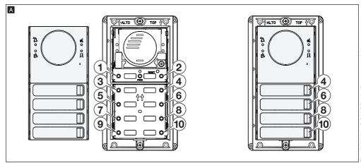
Each group can be associated with a call key (see chapter 3. Associated a user group to a call key on the entry panel). The numbering on the keys follows the logic illustrated in the figure A, according to which key 1 is associated with the group 1, key 2 to group 2 and so on. A call order is associated with the telephone numbers that compose groups, and that call order is used to handle the call rerouting in case there is no answer B.
