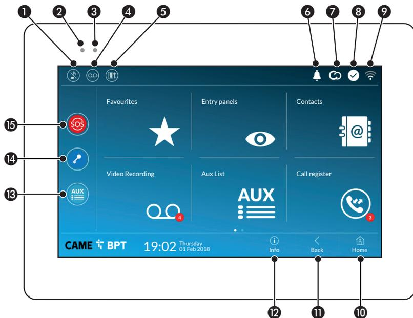
**1** Command to exclude call ringer; when the command is active, the red LED is lit.
