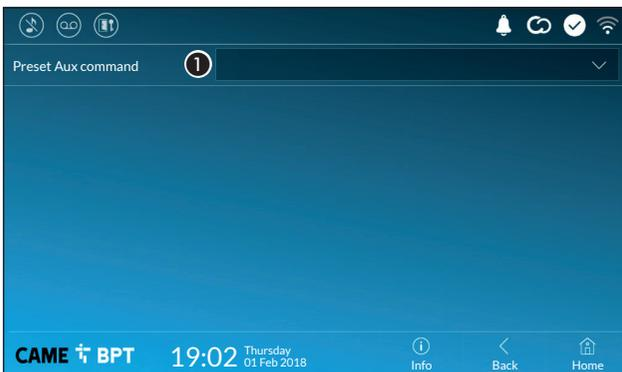
This window is for establishing which of the previously configured commands needs to be executed by pressing the Aux button on the homepage.
