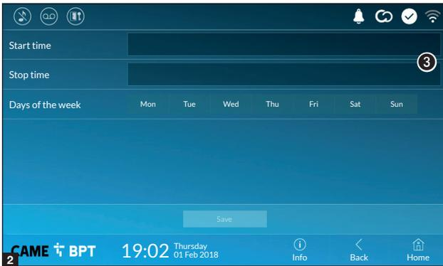
3 Touch the empty sections and in the pop-up window set the start and finish time of the time-slot for activating the function.
