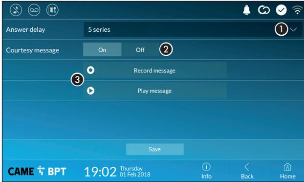
1 From the drop down menu, select the ring time - expressed in seconds - after which the automatic recording is activated.
