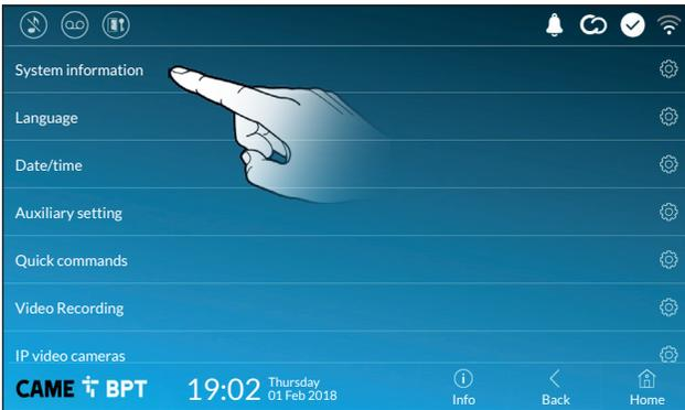
This window gives technical information that is useful for identifying the device's characteristics and the hardware and software versions.
