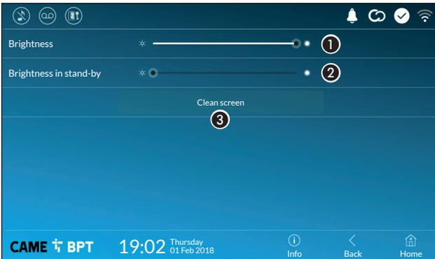
1 Adjusts the brightness of the screen during use.
