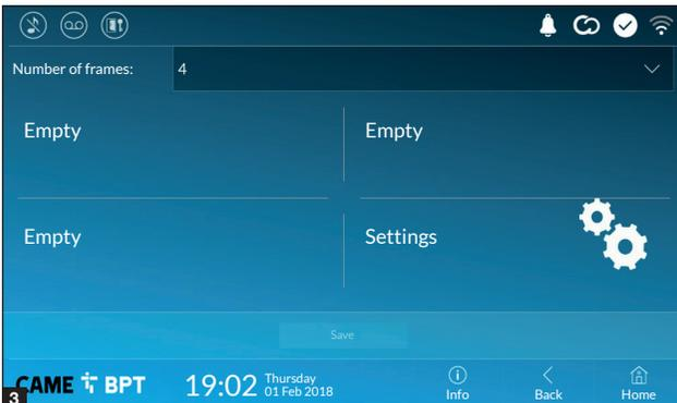
Touch each of the empty sections and use the drop-down menu to select the content that you want to assign to the section.
