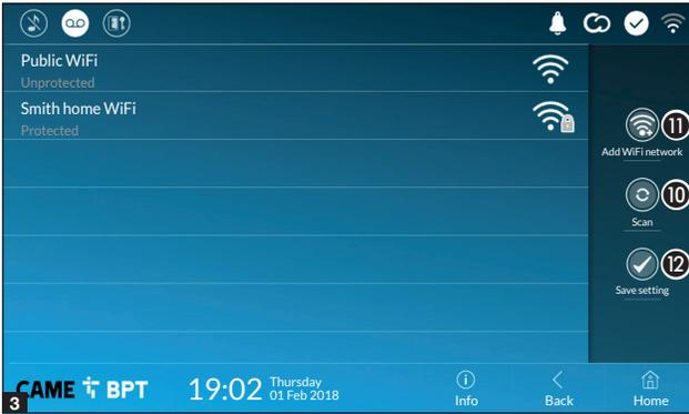
3 The page shows the detected networks; to manually scan for networks, touch the 10 button.
