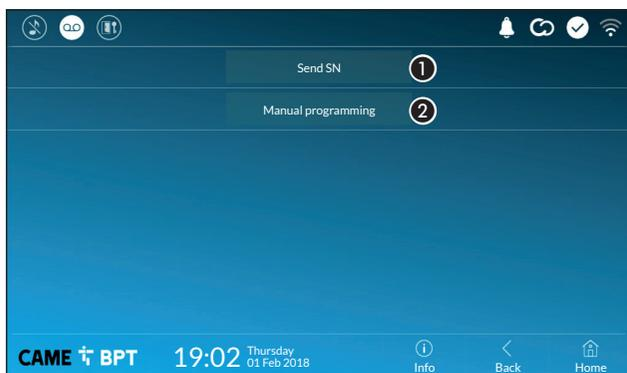
**1** This button is for sending the SN (serial number) to the Pcs/Xip software during the programming steps.
