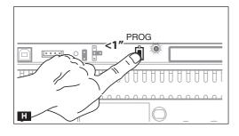
Press the PROG button briefly **H**. The LEDs on the entry panel switch off.
