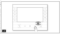
While programming the calls, the "visual range" of the video camera can be adjusted from any receiver. To do this, lift the handset (where present) and press the "self-connection" © button J.
