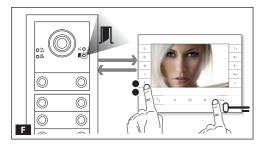
The green LED **□** flashes. Lift the internal receiver handset (if present) and press the door lock release 0—and AUX2 buttons **□**.
