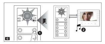
On the entry panel, press the call button to be linked to the internal receiver • 1. A beep confirms that the setting has been stored • 2. End the call and repeat for the other internal receivers.
