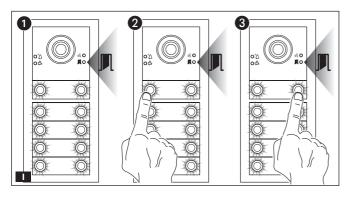
During call programming , you can control the brightness and colour of the unit backlight. Press the left call button to select white , and the right call button to select blue .
