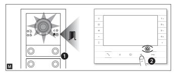
While programming calls **M** 1 the brightness level of the entry panel can be adjusted from any receiver. Pressing the "self-connection © " button on the internal receiver **M** 2 activates the video camera on the entry panel for which the brightness level is to be adjusted.
