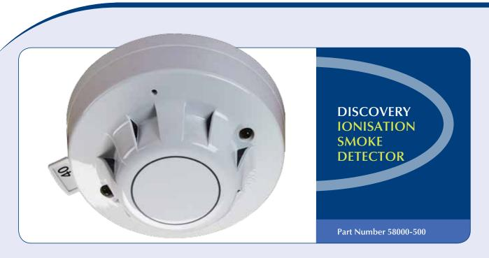
The Discovery Ionisation Smoke Detector uses the same outer case as the optical smoke detector and is distinguished by the red indicator LEDs. Inside the case is a printed circuit board which has the ionisation chamber mounted on one side and the signal processing and communications electronics on the other.
