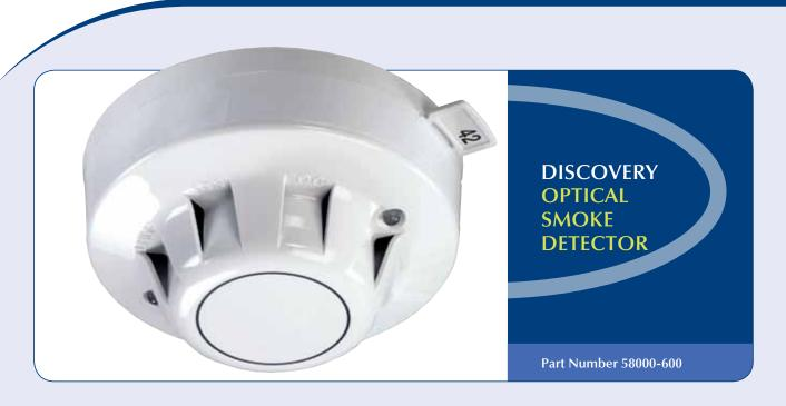
The Discovery Optical Detector has a white moulded polycarbonate case with wind-resistant smoke inlets. The indicator LEDs are colourless when the detector is in quiescent state and red in alarm. Within the case is a printed circuit board which, on one side, has the light-proof chamber with integral gauze surrounding the optical measuring system and, on the other, the signal processing and communications electronics.
