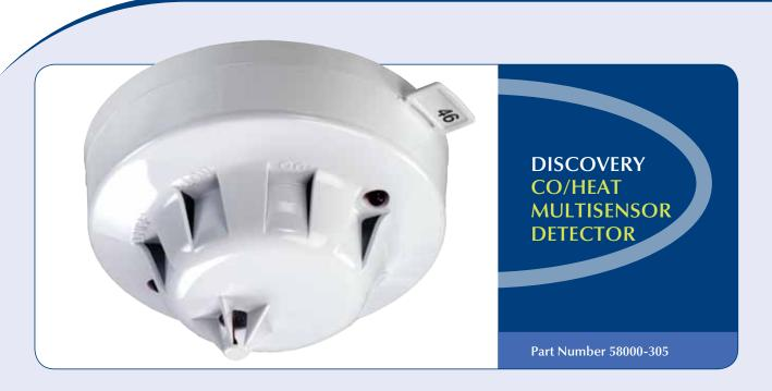
The Discovery CO/Heat Multisensor Detector contains a CO detection cell and a thermistor temperature sensor whose outputs are combined to give the final analogue value. The way in which the signals from the two sensors is combined depends on the response mode selected. The CO/Heat Multisensor detects the presence of carbon monoxide or heat or a combination of both.
