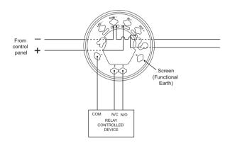
Fig 2 Relay base wiring connections
