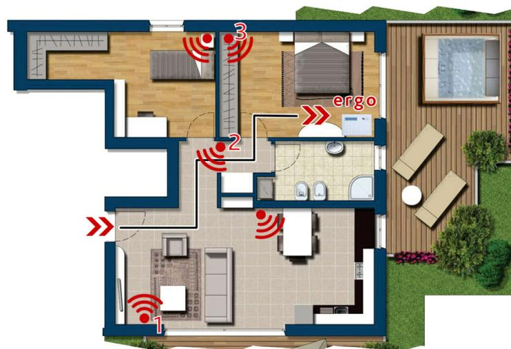
The figure shows a hypothetical situation of entrance into a house where the control panel of the system can be reached only after having intercepted some areas. Specifically, the volumetric sensor marked with ( 1 ) must be the first to be violated so as not to generate an alarm. Then, the number (2) and the number (3) will follow.
