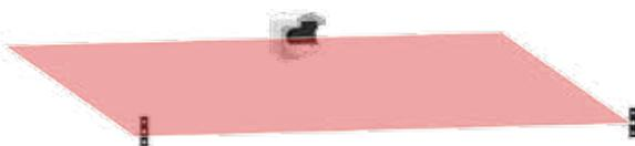
Instruct a person hold the LAC-1 and stand at either side edge of required protection area. The person should hold LAC-1 in front of their body between shoulder and hip line.
