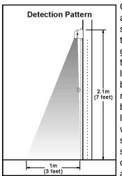
Once the T.REX is installed and the cover replaced, the span and target direction of the detection pattern is set by gently turning the louver direction screws, located just below the detector lens on the barrel. As the adjustment range is about 45°, you must be careful not to turn the louvers too far; stop turning when resistance is felt. The slots on the louver adjusting screws indicate the position of the louver and serve as an adjustment guide. To adjust
